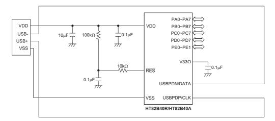
Note: The resistance and capacitance for the reset circuit should be designed in such a way as to ensure that the VDD is stable and remains within a valid operating voltage range before bringing RES high.
