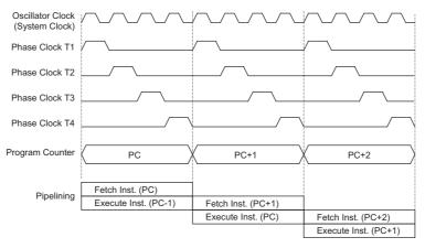
**System Clocking and Pipelining**
